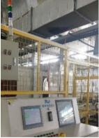
Upgrade of safety protection for engraving and milling machines and extruders. Main electrical control systems have been reconfigured and placed outside to reduce risks in operation and programming
