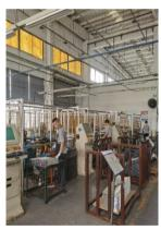
Electrical control parts of single and double bending machines and stamping machines moved to the outside of the protective fence to lower risks in electrical control systems during inspection and maintenance
