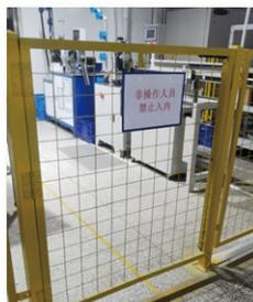
**Linked protection door:** Installing linked protection door(s). All equipment will automatically stop running when the linked protection door is opened.
